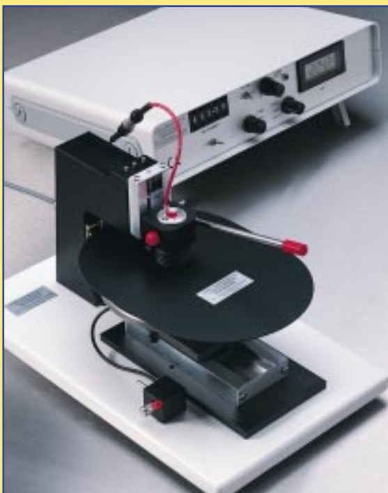
Measuring system comprising a Multiposition Probe and Test Unit.
