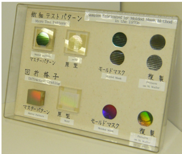
Fig. 17. (Color online) Samples fabricated by molded mask method in the 1970s. From left to right: master pattern, mold, molded mask, and pattern fabricated on Si wafer substrate. Top: microsized test pattern. Bottom: diffraction grating.
